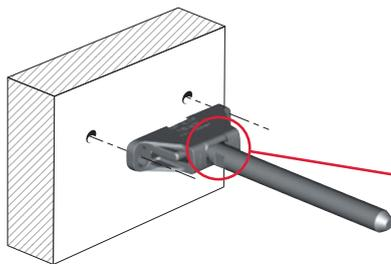
Recommended fixing pan head screw type - head Ø 5 mm max.
