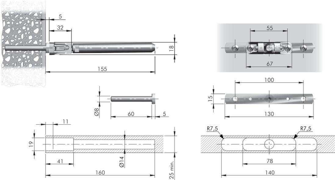
**TRIADE MINI BRACKET FIXING ACCESSORY**
